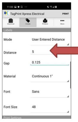
6. In the example below, distance has been changed to 5". Material is Continuous 1" by default but can be changed by tapping the field to see other options. When ready, select PRINT.
