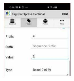
Select PRINT when ready. You can reverse the print by printing the largest number first, for use in Data Centers and Patch Panels, or leave as is for terminal block marking.
